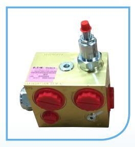
Hydraulic flow divider valve works on all hoist systems. It has a standard aluminum body rated at 3,800 psi and provides flows up to 50 gpm with full relief valve protection.
