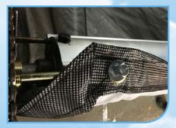
Durable, professionally threaded bolt takes the guesswork out of attaching the tarp.
