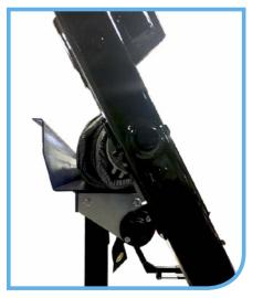
Upper extension arm makes it easier to preload the spring roller and minimize the potential for the tarp roller shaft to seize in the arm bushing
