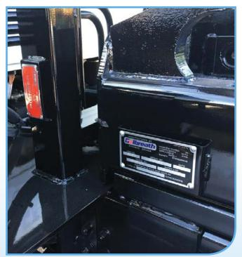
Riveted-style serial number plate allows for permanent identification of a unit
